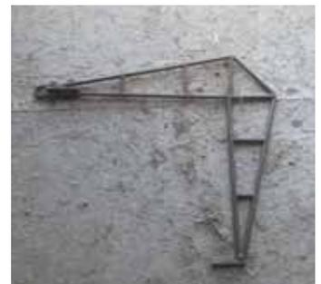
Bale hook is a right angle device reinforced with roof truss-like supports.
