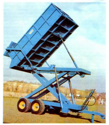
Height of 9-ton Warwick high lift tipping wagon is infinitely variable up to 11 ft., 9 in. Box can be tipped (to full 55°) for fast unloading at any height. Twin 3-stage cylinders do the lifting, and another 3 stage cylinder the tipping.
