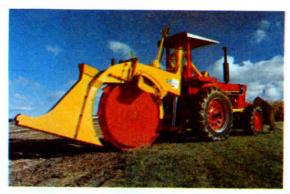
Tractor pto drives trencher. Digs trench up to 12 in. wide and 5 ft. deep. Large wheel (7 ft., 3 in. dia.) is the only moving part. Lays plastic or clay tile at rate of 30 to 50 ft./min.
