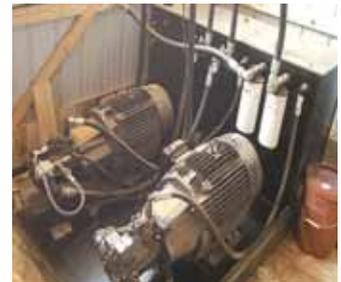
Control panel is located in center of U near baler (left). Bale Converter and Bale Baron operate on hydraulic pumps powered by two 3-phase electric motors
