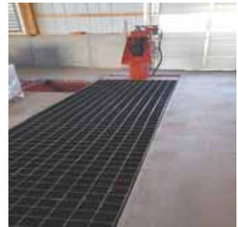
System includes 90 ft. of in-floor augers covered by steel grills. This one feeds chaff from Bale Converter to baler.
