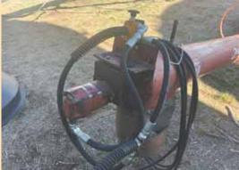
Hydraulic directional valve mounts on top of an auger Pfaltzgraff uses to unload semi trucks. "I just press a button to shut off the auger. It saves a lot of walking," he says.
