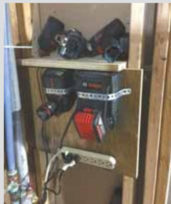
**Jack Middleton, Marquette, Mich.:** “I didn’t like having the bench space in my shop cluttered with battery chargers for my cordless tools, so I used plumber’s strapping to attach the chargers to the shop wall. I place the cordless tool on a shelf while its battery is being charged and plug the charger into a power strip that I installed below the shelf. I can easily shut the power off to the charger whenever it’s not in use.”
