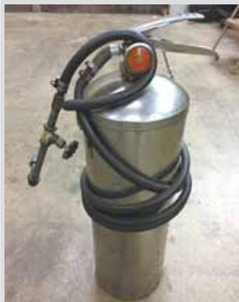
**Jon Arms, Brewster, Mass.:** “I use a surplus fire extinguisher to add gear oil to gearboxes. I fitted it with a pressure hose and a 1/4-in. nip valve. It holds about 2 gal. of oil, added through the top nut that holds the handle and dip tube. Air is added through the snifter valve at the top beside the pressure gauge.
