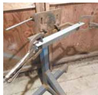
Modified engine stand allows Bontrager to rotate pieces as he welds.
