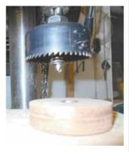
Releasing pressure on drill press causes spring to automatically push donut out.
