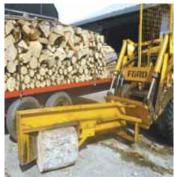
Log splitter is built from 2 pieces of channel iron mounted back to back, with a "window" in between. It can handle wood chunks from 4 to 20 in. in diameter.
