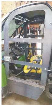
Home-built doors have bolt-equipped gate hinges that fit into Gator's door hinges. "To remove a door, I just lift it off," says Ken Veach.
