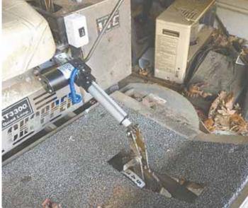
Ed Clayton wanted to raise the deck on his zero-turn mower without having to push down hard on the pedal, so he replaced it with an actuator kit mounted below the seat.
