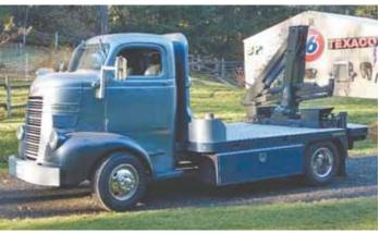
Charlie Brown converted an old Dodge COE semi truck into this shop truck complete with a flatbed and knuckle boom crane.
