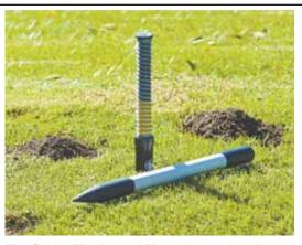
The GopherHawk trap kills gophers and moles immediately without the use of poisons or bait (left). The three-pronged, stainless steel snare and trigger are exposed in the tunnel when the trap is engaged (above left). A probe and wedge tool is used to find the tunnel and make a hole into it (the thin probe stores inside the wedge). Then the trap is inserted in the hole vertically. The yellow stripe indicates the trap has been triggered (above).
