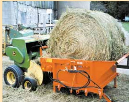
Machine unwinds bale directly over pickup reel of any small square baler. You can see a video of the Altec bale unwinder at our YouTube channel: “[thestgeorgeco](http://www.thestgeorgeco.com)”.
