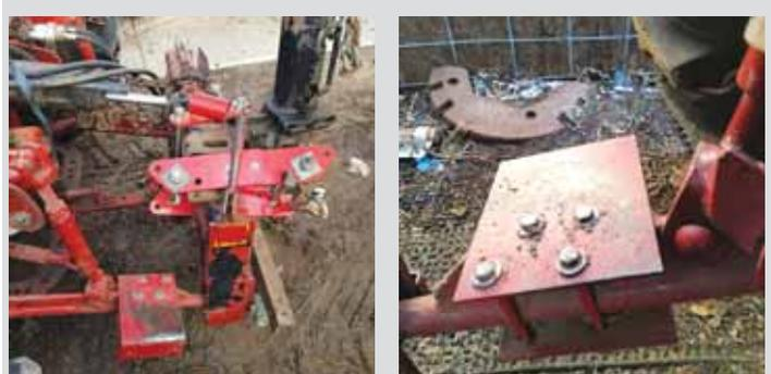
U-shaped steel plate bolts onto 3-pt. lower lift arm, making it safer to climb up onto tractor.
