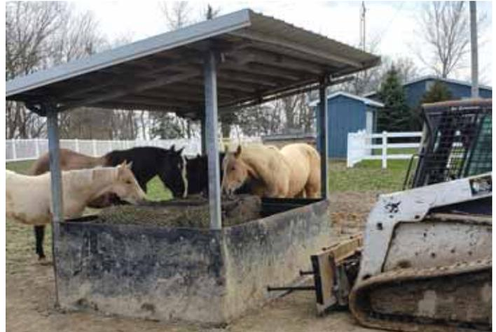
Portable big bale feeder is built entirely from steel and used rubber belting. Skid loader’s bale spears fit into a pair of metal tubes to pick up feeder.
