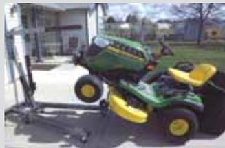
**Jim & Ruth Hopkins, Nampa, Idaho:** "We use our portable engine hoist to lift the front end of our garden tractor to easily remove blades for sharpening and to clean under the deck. Also makes it easier to lube. Helps us keep the mower in good running condition."
