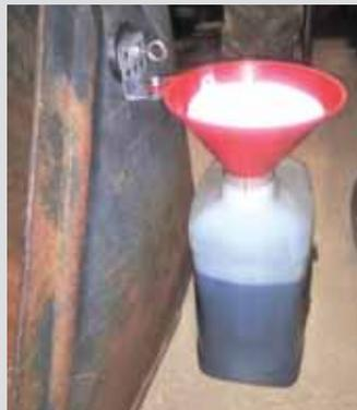
**Glenn A. Halley, Andover, N.H.:** Glen got tired of funnels falling over when pouring in used oil into jugs or handling other fluids. "I attached a round magnet to an angle bracket with an eyebolt. Then I attached the funnel to the leg of the bracket with a small bolt and washer. I can stick the magnet to any metal surface, holding the funnel tightly in place over the jug. Very handy."
