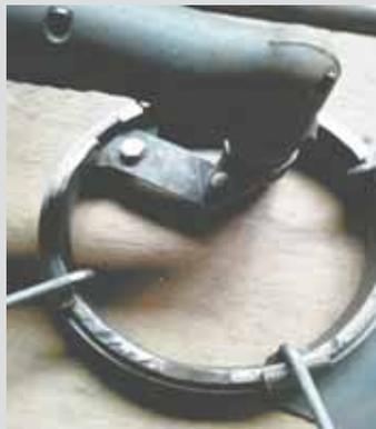
**Carman Fedele, Tidioute, Penn. (ph 814 730-9377):** Carman has a simple solution for cutting perfect circles in metal. His patented torch guide makes it easy. Just clamp down a shoulder plate, insert the torch, and rotate. "My prototype can cut out any size circle up to 4 in. in diameter. You can use it to cut out any size washer needed or cut a perfect hole in a piece of metal."
