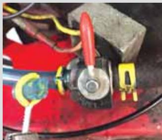
**Cal Miner, Willmar, Minn.:** "Older fuel lines are a larger diameter than newer push-lock type hose. To use newer hose on an older engine, the old clamps won't work. I made my own using an eyebolt. Just cut off the screw part, slide the clamp in place, and squeeze the 'eye' together to clamp it tight. Works great and holds well."
