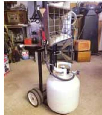
Home-built hand cart makes portable propane heater easy to move around.
