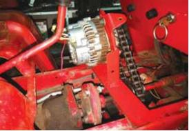
Heron equipped his Cub Cadet with an external alternator off an SUV, replacing the alternator pulley with a sprocket that's chain-driven off the transmission driveshaft.
