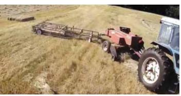
The 10-bale Hay Accumulator turns 2 bales sideways, then adds 2 sets of 4 bales lengthwise. Alternating the 2 odd bales makes trailer load more stable.
