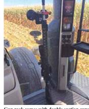
Gun rack comes with double suction cups that grip the glass. Gun barrel fits into a U-shaped rubber pocket on holder.
