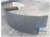
Tabs on steel plate are held in place by mower's spring-loaded discharge chute.
