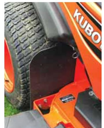
Rubber mud flaps bolt on ahead of mower’s rear wheels to keep deck clean.
