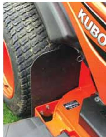
Rubber mud flaps bolt on ahead of mower’s rear wheels to keep deck clean.
