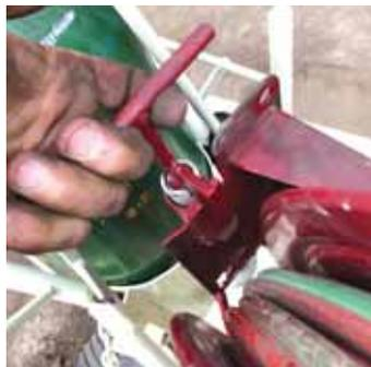
Spring-loaded T-bar rides in a slot on hose reel hinge plate to hold reel in place.
