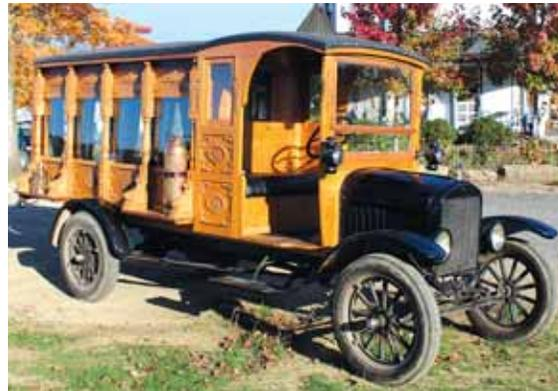
Old-style hearse was built on a 1925 Ford Model TT cab and chassis, and has decorative moldings on the sides along with an antique fire extinguisher.
