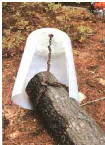
**Log is secured by a choker chain that runs through hole in bottom of plastic cone.**
