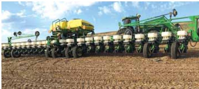
**Bolt-on Fat Cat Tire system nearly doubles tire contact with the soil, helping to fight pinch-row compaction caused by large, heavy planters.**
