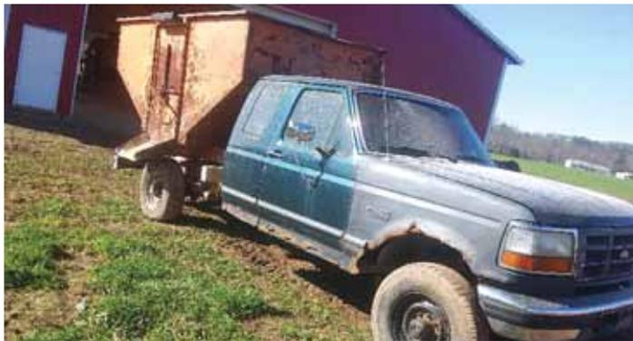
Peter Donnelly built this feed truck by combining parts from a Ford F-350 pickup and an old gravity wagon box.
