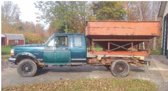
He bolted a pair of 6 by 6 wood beams onto the pickup frame, then bolted the hopper onto it using original mounting brackets.
