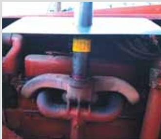
**Gary Swensen, Yankton, S.Dak.:** “My old Farmall has a cracked exhaust manifold. When it was out in the rain, water would get into the engine. So I came up with a quick fix until I have time to fix it permanently. I cut a hole in a heavy piece of sheet metal and slipped it over the exhaust pipe. The sheet metal fits tightly so it keeps water out. It’s hidden under the hood so it doesn’t change the look of the tractor.”
