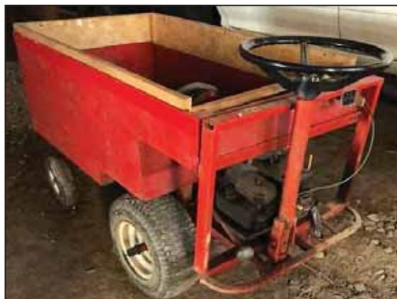
Motorized, walk-behind "sweet corn cart" was made using parts from a pair of riding mowers. Operator pulls back on steering wheel to propel cart forward.
