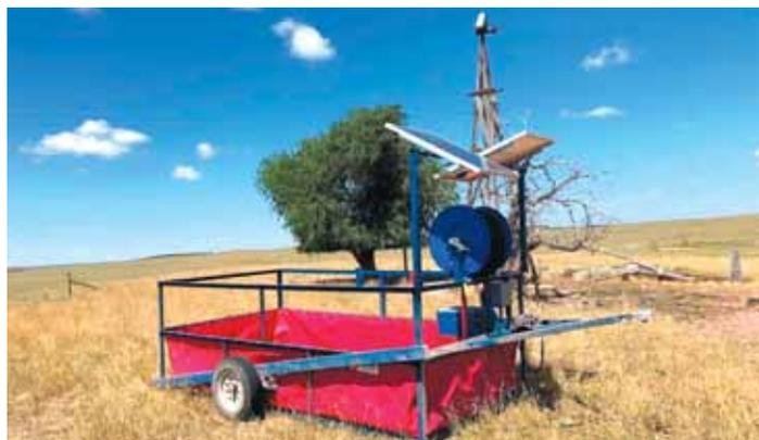
Mobile water tank mounts on its own trailer and comes with a float system and optional solar-powered pump.
