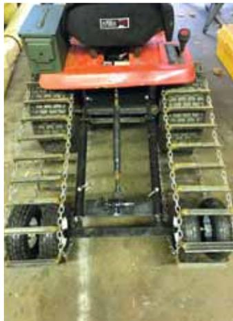
A pair of telescoping shocks keep down pressure on the bogie wheels and allows tracks to move up and down freely. Tractor's front wheels can be fitted with snowmobile skis held on by ratchet straps.
