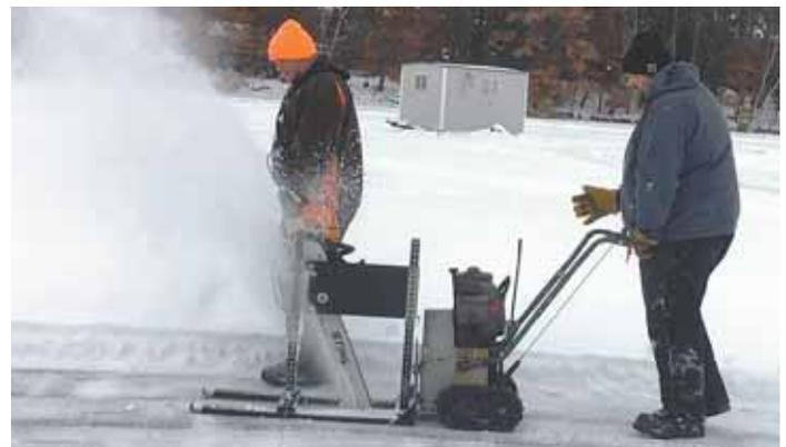
To cut the ice they use a chainsaw secured on a “Chainsaw Chariot” built out of a tracked snowblower.
