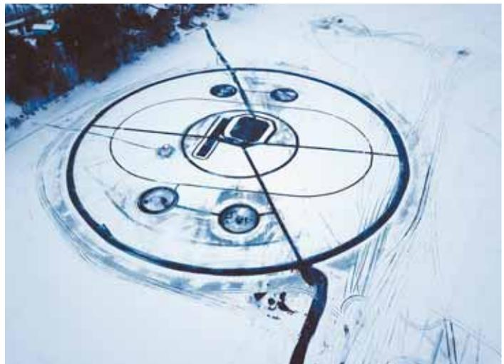
Giant powered ice carousel measures 508 ft. in dia. and is rotated by 4 electric trolling motors. Four smaller carousels were cut into the big one.
