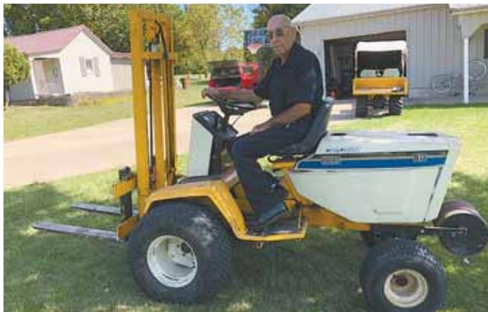
Birkey turned this Cub Cadet into a forklift, reversing the steering, seat, and controls and flipping the ring gear and pinion in order to operate the tractor backward.
