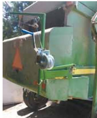
Boat winch is used to swing roll sideways over into baler's storage compartment.
