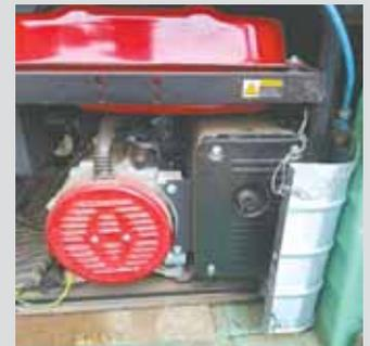
**Gary Swensen, Yankton, S. Dak.:** "I carry a generator in the back of my 2004 V-10 Ford pickup and needed a heat shield to protect the paint on the side of the box from muffler heat. I bought a metal basement window protector for \$10 at Menards and wrapped it around the side of the generator. Does the trick."
