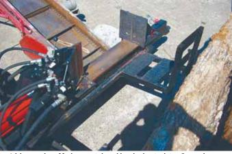
Les Adelman and son Mark converted an old grain elevator into a firewood conveyor. A 5-speed transmission off a Ford Pinto lets them gear the conveyor down as needed.
