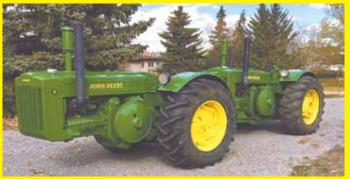
Thanks for showing my John Deere Tandem "D" tractor in your last issue. I'm considering selling this tandem tractor, which I put together in 1966. The back tractor is a 1947 D while the front one is a 1949 D, both with electric start. I needed more power to pull bigger equipment and they weren't making big 4-WD's at the time.
