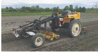
Reid Allaway replaced the Renault engine on his Hefty-G cultivating tractor with an 8-in. dia.  $\overline{DC}$  motor and controller off old forklifts.
