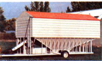
The 1,250-bu. portable field storage tank has its own self-contained hydraulics that power the bin's 10-in. loading auger, 12-in. unloading auger and 7-in. leveling auger.
