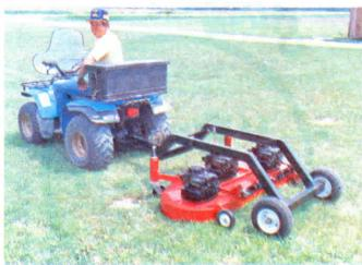
Mower height up to 3 in. is controlled by cranks on the caster wheels. From 3 to 12 in., mower height is controlled by a hand-cranked cable winch on the tongue.
