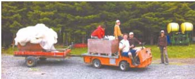
Reid Allaway rebuilt this electric-powered warehouse truck to use on his vegetable farm. "It has ample power to haul a trailer or heavy loads," he says.
