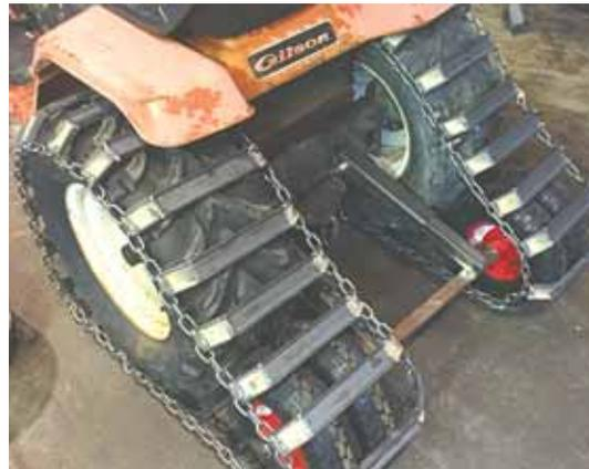
Harry Dykstra uses his half track garden tractor to build trails in his woods and haul out firewood without making wheel ruts. Four 8-in. tires on back serve as "dolly wheels" for the tracks.
