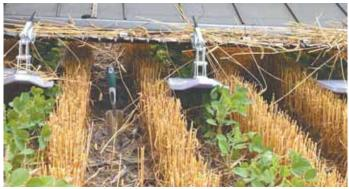
FlexxiFloat "bean shields" hold bean plants down so combine header's knives don't Bean shields bolt to spring-loaded crop lifters that attach to header. damage them. Once the header has passed over, plants pop back up.
