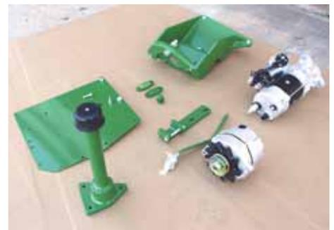
Photo shows Horning's electric start kit for Deere 830 and 820 tractors. All kits are sand-blasted and painted.
