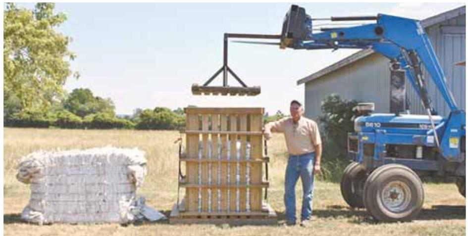
Lynn Leavitt with his “Pac-it” bale wrap compactor. Plunger attached to front-end loader compresses plastic as it’s added to wooden box. Tied-off plastic bale is shown at left.
