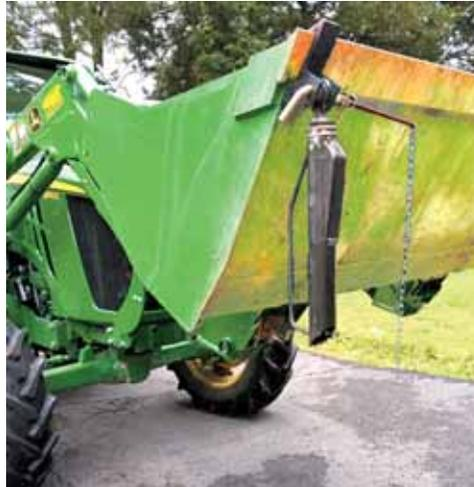
Tee-Post driver hangs from loader bucket. Post slips into driver barrel, which swings freely on swivel, allowing gravity to align posts. By inserting a pin to lock onto fencepost notch, posts can be pulled quickly with driver.
