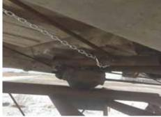
Up to 3 people can sit on the roomy, full-size pickup seat. The end drive gearbox off an old center pivot irrigator serves as the turntable mechanism for the cab.
