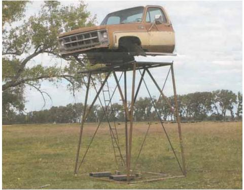
Austin Roney made a rotating deer stand by mounting a pickup cab on top of a metal stand. Cab rotates 360 degrees on a turntable mechanism.
