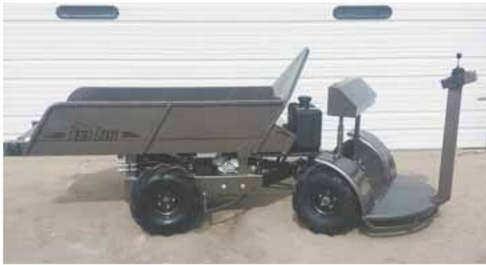
Developed for use in large turkey barns, the Barn Boss has a standing platform with a joystick control on front, followed by a "live box" with an apron chain.
