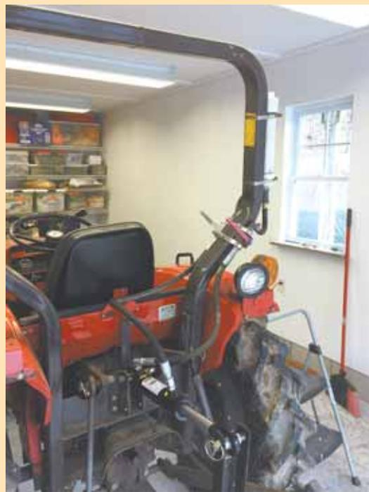
Medley mounted a hydraulic cylinder in place of a standard 3-pt. top link, and ran hoses from the cylinder to 2 high-pressure ball valves and a reservoir mounted on his ROPS.
