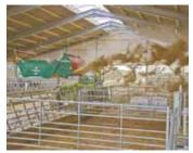
Telehandler equipped with BFR-180's Crossfire straw spreader attachment (above) throws baled straw to use as bedding. A sidewinder attachment feeds bale into a trough (below).
