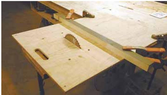
Paul Tierney used his hand-held circular saw to cut a slot into a sheet of plywood, then set the saw over the slot with the blade sticking through it. He bolted the saw's baseplate to the plywood and then flipped the plywood over so the blade extends out the top.
