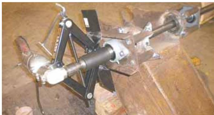
Brian Lough needed to enlarge the bore of the pin holes on his 12-in. used excavator bucket, so he built his own line-boring machine. He uses a scissor jack to align it and apply pressure.
