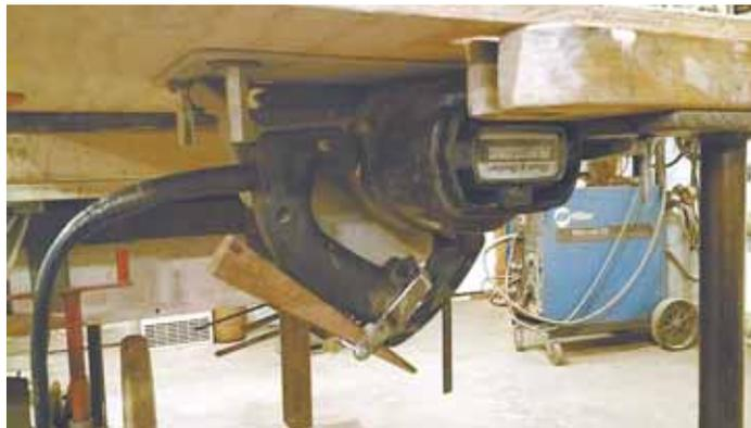
To keep the saw running continuously, he wrapped a metal bracket around the trigger and slipped a small wood wedge under it. To stop the saw, he just pulls out the wedge.
