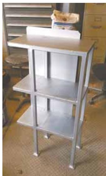
Chainsaws are stored on one side with oil and fuel cans on the other side. Chainsaw bars extend through gap at the back.
