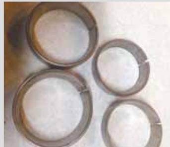
**Warren Grant, Albany, Ga.:** “I’ve always had trouble pushing new races back into place when a bearing goes bad. To solve the problem, I take a Dremel tool fitted with a small cut-off blade and cut through one side of the old race. It makes the race flexible enough that I can push a new race in and then remove the old one with little effort. Every time I change out a race, I save it so that I’ll have various sizes on hand.”
