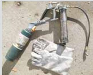
**Gary Swensen, Yankton, S. Dak.:** “In the winter it can be almost impossible to pump grease when it’s cold and the grease gun is left outside. I solve the problem by heating the grease gun up with a torch for a few seconds, which gets the grease flowing like summertime. Just make sure to wear welding gloves since the gun can get really hot.”
