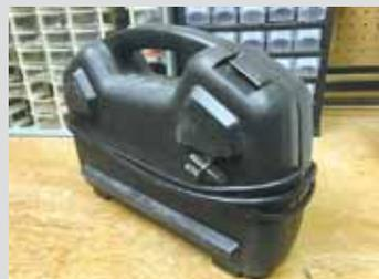
**Ryan Van Der Bill, Sioux Falls, S. Dak.:** “Instead of trying to stuff a tool’s electric cord inside the tool case box, just wrap the cord neatly around the outside of the box. You might have to cut a small groove in the plastic where the box folds up in order to run the cord through.”
