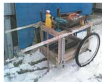
Tool cart rides on bicycle tires mounted to a frame built from broken pallets, with hockey sticks for handles.
