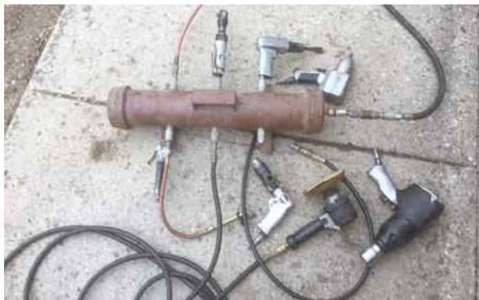
Mobile air splitter is made from a large heavy-gauge pipe with ends welded in place, and holes drilled in the sides to connect air lines.
