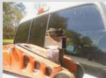
**David Norman, Bay St. Louis, Miss.:** “I keep hydraulic floor jacks in 4 different pickups. I gave each jack an extra 2 in. of lifting height by welding a 4-in. length of 2-in. square tubing onto it. I removed the pin that secures a steel cup to the jack lift arm and welded the tubing on. Then I drilled a hole in the tubing, placed the cup on top of it, and reinserted the pin.”
