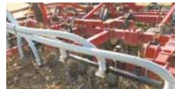
Manifold and distribution system uses 12 hoses with seed deflectors on their ends.
