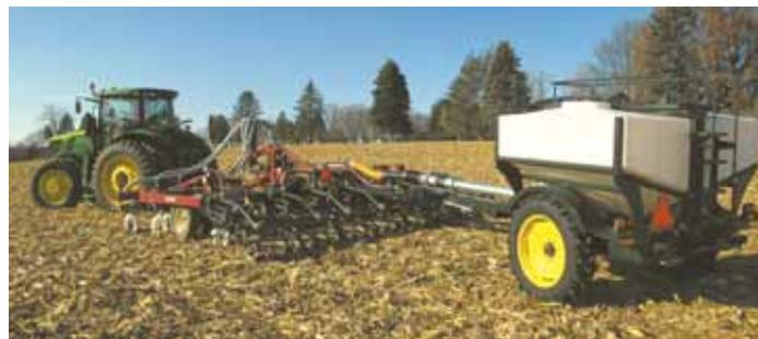
Verti-Seed Cart converts field cultivators, disks and other tillage toolbars into cover crop seeders that can till and seed in one pass.
