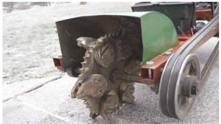
He bolted 12 Rayco stump grinder teeth onto a 48-tooth, no. 60 chain sprocket that's belt-driven off mower engine.
