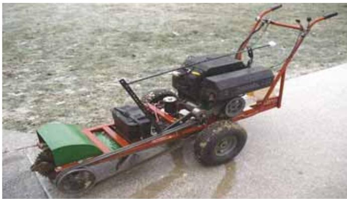
Kenny Ranta built this self-propelled stump grinder out of an old Cub Cadet riding mower and the handlebars off a walk-behind rototiller.
