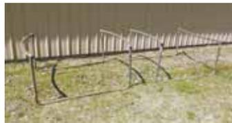
He reassembled the slip joint pieces on one trampoline to use as sawhorses, topping them with plywood.
