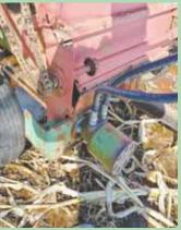
Gears driving the conveyor on his front unloading silage wagon wore out, so Wimmer removed them and bolted an orbit motor directly to the conveyor driveshaft.
