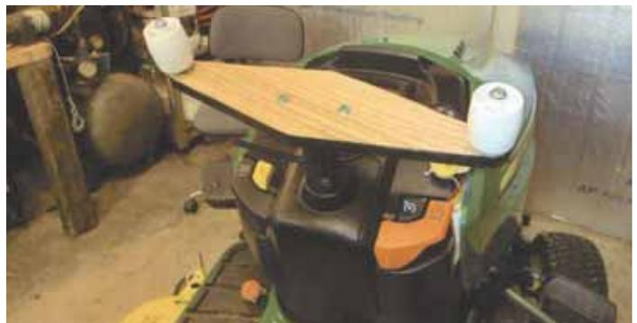
To make it easier to get on and off his garden tractor, H.T. Kuyper replaced the factory steering wheel with an oak crossbar and put caster wheel knobs on each end.
