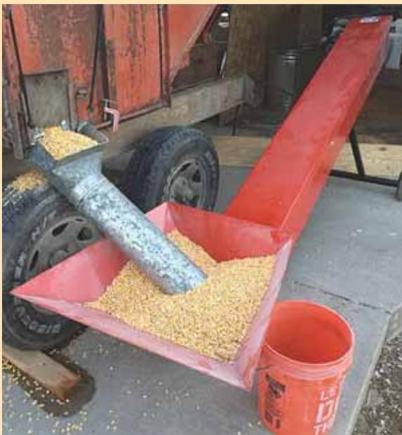
Beans feed into roaster from hopper at one end and slowly travel up an electrically-heated oven chamber. They exit near the top end fully roasted.
