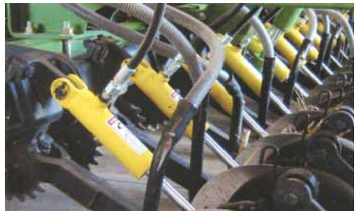
UniForce hydraulic down pressure system is designed for Deere drills. Single-action cylinders on each opener keep down pressure constant on uneven ground.
