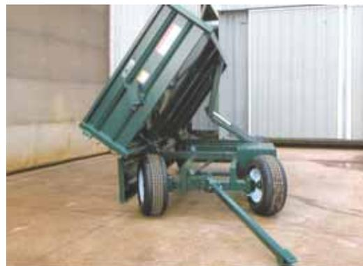
Side dump trailer is built with a scissor lift for quick unloading. Both axles steer for great maneuverability.
