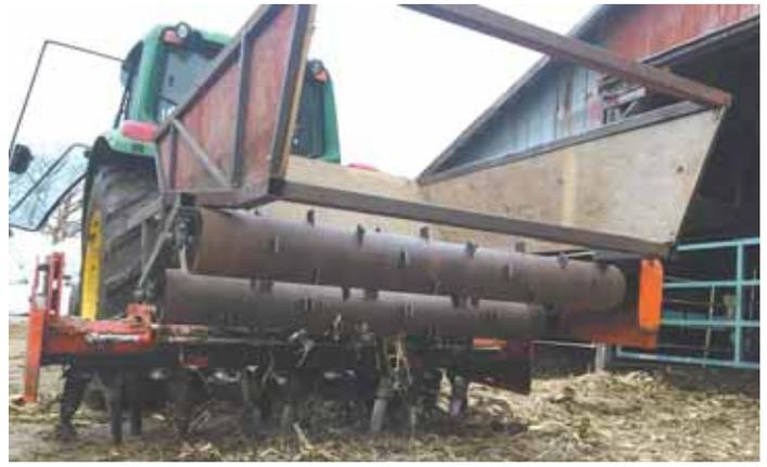
Unroller was built by welding 2-in. steel fingers onto two 8-in. dia. rollers and building a frame to hold the bale.
