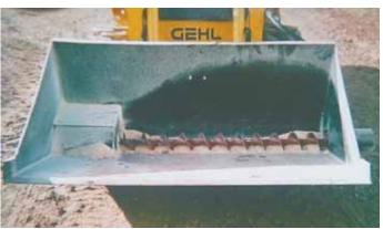
Home-built skid loader bucket is equipped with an auger and side chute that makes filling feed bunks an easy job.
