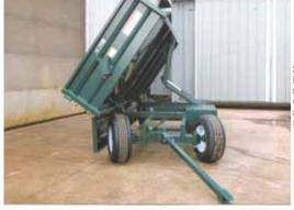
Side dump trailer is built with a scissor lift for quick unloading. Both axles steer for great maneuverability.
