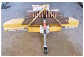
Boat trailer jack mounted on grader hitch makes 3-pt. hookup easy.
