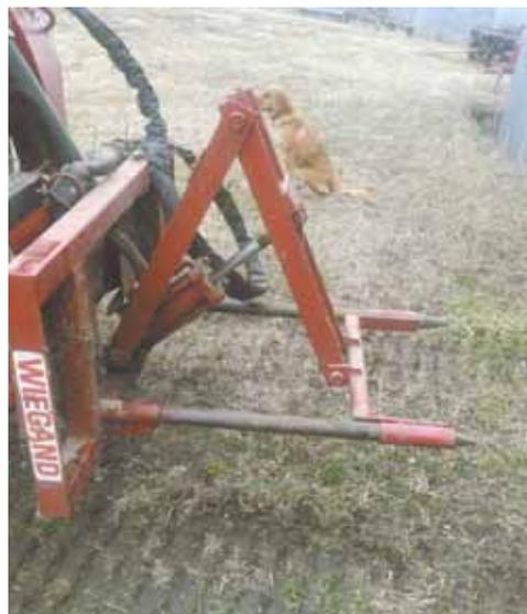
Scissor-action push bar slides big round bales off, no matter the angle of the bale lifter spears.
