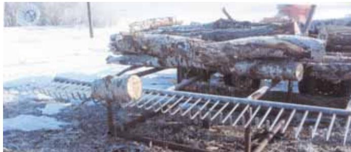
A 12-ft. pipe across front of stand has steel rerod fingers welded to it every 4 in., with their ends bent upward to keep logs from rolling off.
