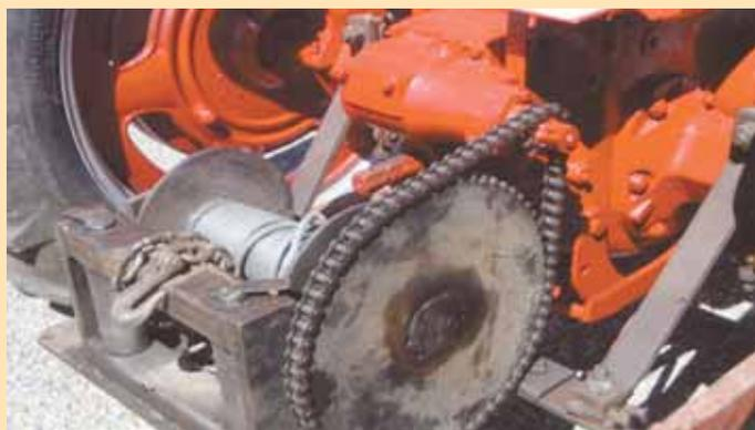
Winch spool assembly bolts to Farmall's drawbar and is chain-driven off tractor's belt pulley driveshaft.
