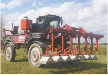
Shuter Farms uses hot water to kill weeds on contact. Their diesel-fired system includes a water heater, water tank, and 7 hoods and nozzles attached to a Miller Nitro sprayer.
