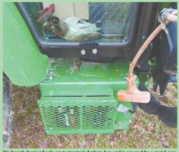
On-board charger hooks up to tractor's battery box and is covered by a metal cage. To charge the battery, Jett pulls out charger cord pigtail and hooks it up to an extension cord.
